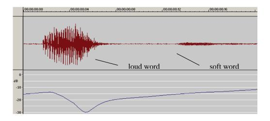
Red waveform is output of hearing aid with a dual time constants. Blue line is instantaneous gain of compressor for this sound. Note that the compressor gain recovers rather slowly after the loud speaker. The gain is at -15dB when the soft word starts.
