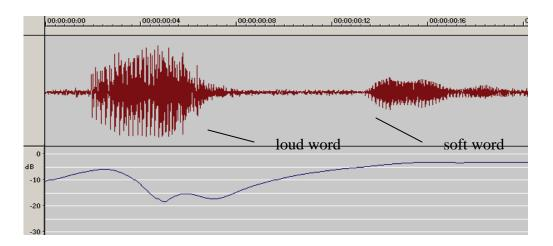
Red waveform is output of hearing aid with Dynamic Contrast Detection activated. Blue line is instantaneous gain of compressor for this sound. Note that the compressor gain recovers more quickly after the loud speaker. The gain is at -5dB when the soft word starts. This is 10dB more gain than without Dynamic Contrast Detection.
