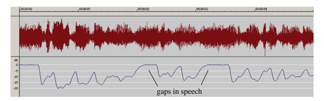
Red waveform is output of hearing aid with a single fast release time of 120 milliseconds. Blue line is instantaneous gain of compressor for this sound. Note that the compressor gain jumps up to 0dB every time there is a gap in the speech. When this happens, the background noise is overamplified, so the noise gets loud every time the speaker pauses.
