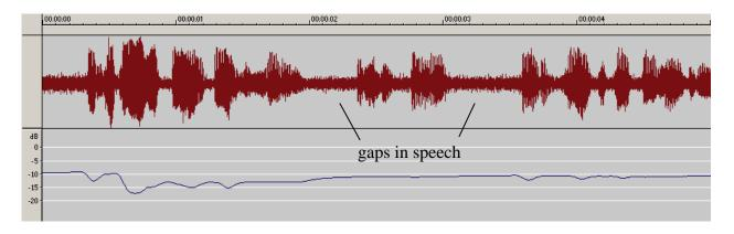
Red waveform is output of hearing aid with Dynamic Contrast Detection activated. For this sound signal, the compressor uses a long release time of 15 seconds. The Blue line is instantaneous gain of compressor for this sound. Note that the compressor gain stays relatively constant through the gaps in the speech. Therefore, the noise stays at low levels when the speaker pauses.
