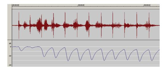
Red waveform is output of hearing aid with Dynamic Contrast Detection activated. For this sound signal, the compressor uses a fast attack, fast release. The Blue line is instantaneous gain of compressor for this sound. Note that the compressor gain recovers between claps. Therefore, the speech gets amplified by about 10 dB more than with the single long release time.
