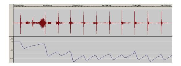
Red waveform is output of hearing aid with a single long release time of 800 milliseconds. Blue line is instantaneous gain of compressor for this sound. Note that the compressor gain drops quickly when
